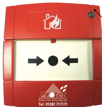
If the Red LED (Light) is illuminated on the MCP, the device has been activated. If it has been activated then reset it in accordance with the instructions supplied with the device.
