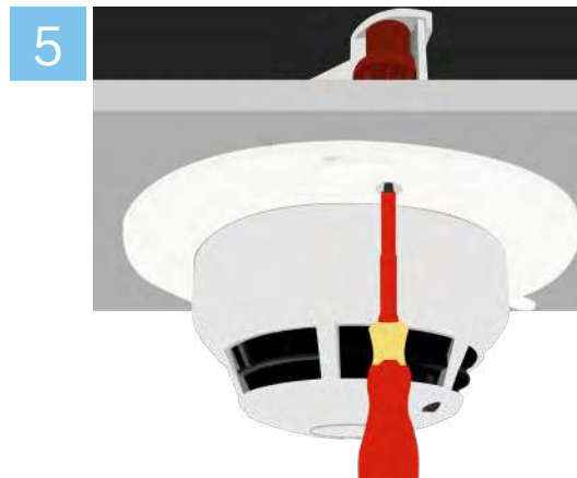
5 Tighten the three detector screws until firmly mounted in position.
