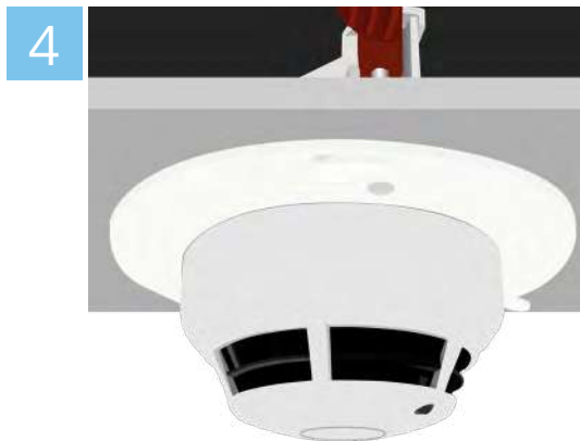
4 Push the detector back into the hole.
