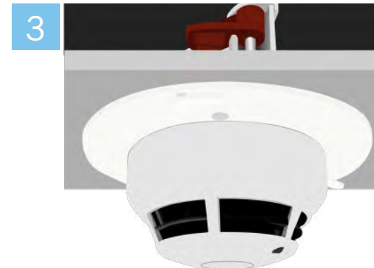
3 Turn the trim clockwise to lock into position.
