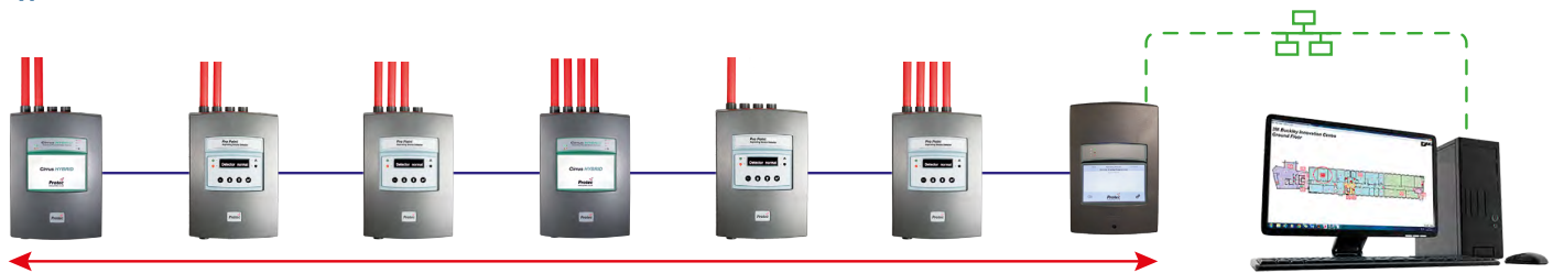
Maximum 98 Protec aspirating detectors on RS485 wired network Maximum 1.2km RS485 network length with one ADRDP (can be extended using multiple ADRDPs)
