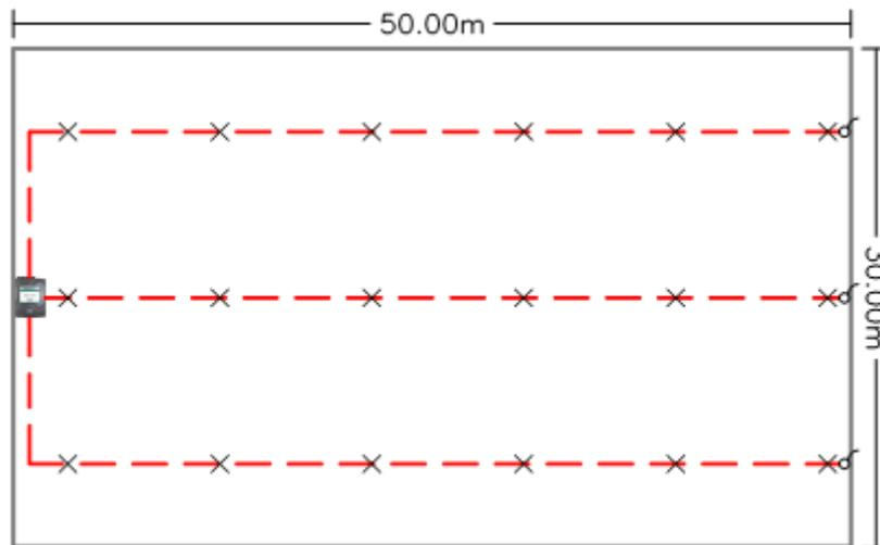
An alternative layout would be to go across the width of a warehouse if this is more suitable. All sampling pipes should be extended to the perimeter wall with low level Maintenance Test points being fitted. Sampling pipes should be supported as per the recommendations of the sampling pipe manufacturer. This method of installation will likely require additional mechanical pipe supports between purlins.
