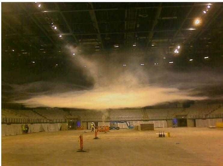
Stratification occurs when air containing smoke particles or gaseous combustion products is heated by smouldering or burning material. Whilst becoming less dense than the surrounding cooler air, it rises until it reaches a level at which there is no longer a difference in temperature between it and the surrounding air. The smoke plume, as it rises, encounters colder air from above which absorbs heat and slows the upward movement of the smoke.
