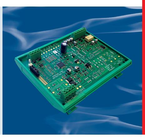
The Protec 2 way loop zone alarm interface is a loop powered input / output device providing 2 local zones of conventional detectors and 2 local monitored alarm outputs.
