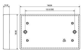
Backbox Requirements - Surface or flush double gang pattress box minimum of 25mm deep.
